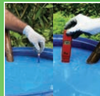
Test the neutrality of the mixture using litmus paper or P H meter
